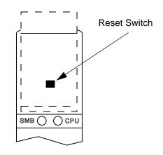
Figure 2-4. The Reset Switch
